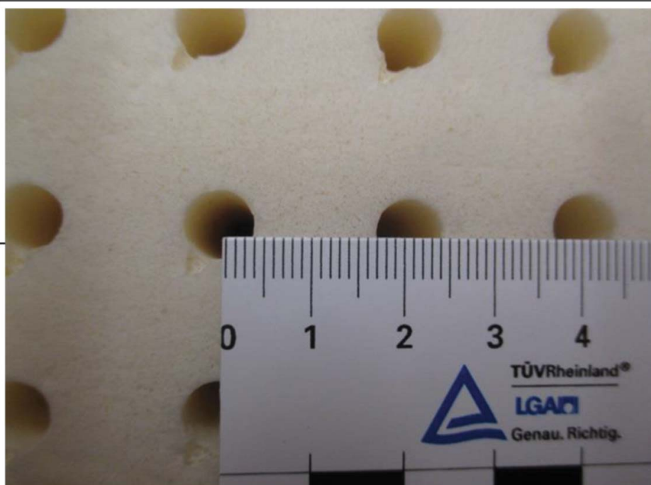
Picture 3: Distance between the holes
